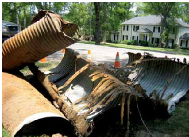
Streets paved recently include Foxwood Road, above. Culverts are showing rust damage after forty or fifty years of use, right. At far right, culvert replacement on Tyne Blvd. preceded paving.
